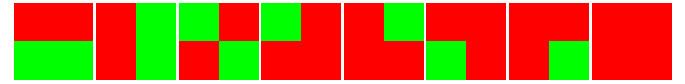
Fig. 3: Eight 2 \times 2 checkerboard-like filters used in this work. Red (Green) is used to represent value +1 (-1).
